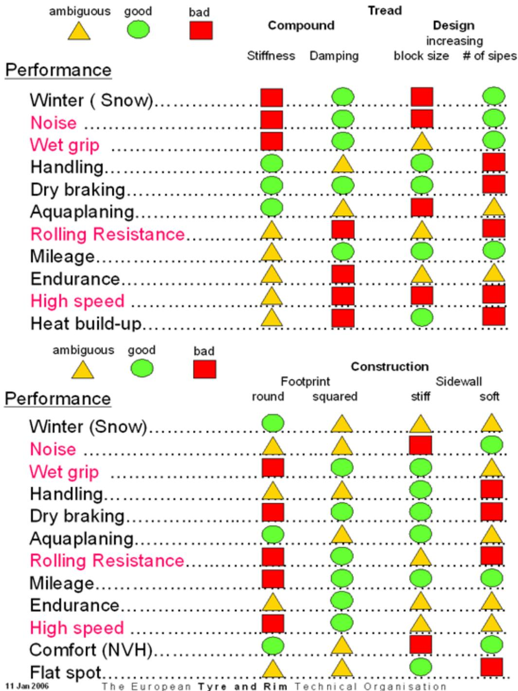
Figure 6-3: Qualitative effect on tyre performance of changing tread parameters (above) or tyre construction (below). Figure submitted by ETRTO to FEHRL, published in [FEHRL, 2006].
