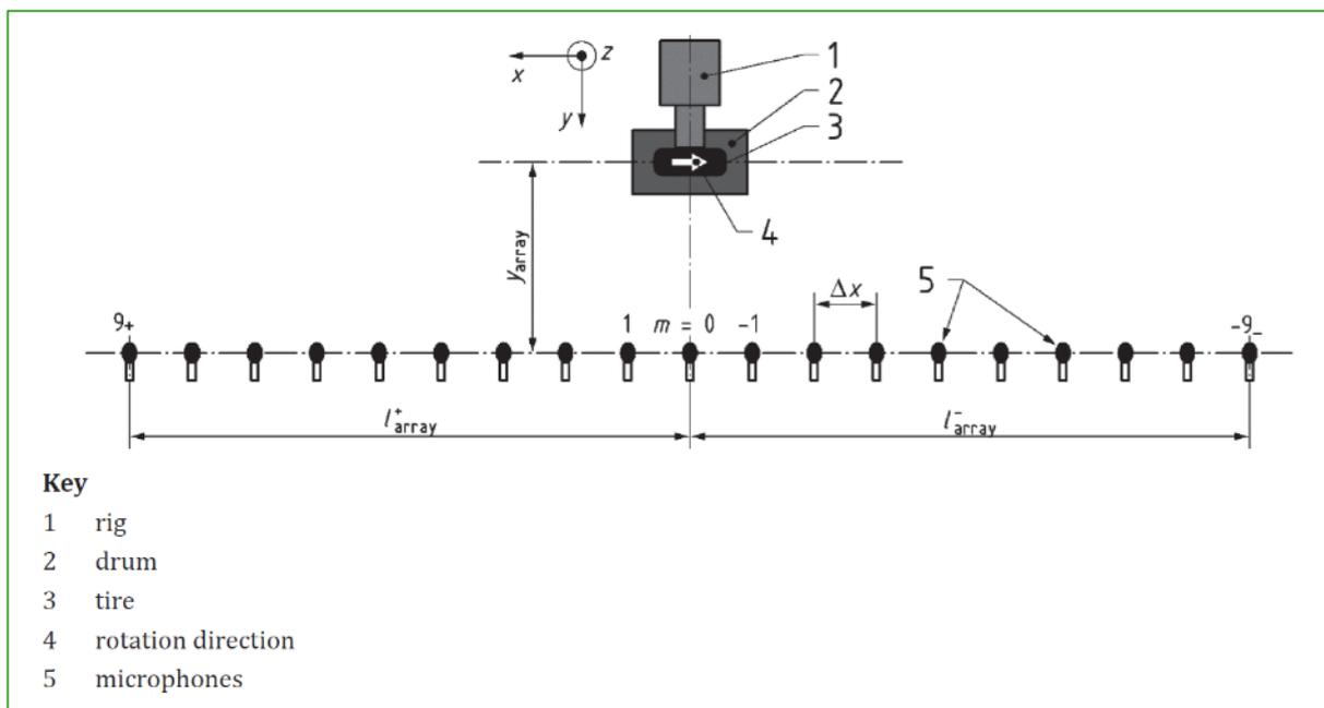
Figure 4-5: Set-up of measurements according to ISO/DIS 20908. The  $Y_{array}$  distance is assumed to be at least 1.75 m.
