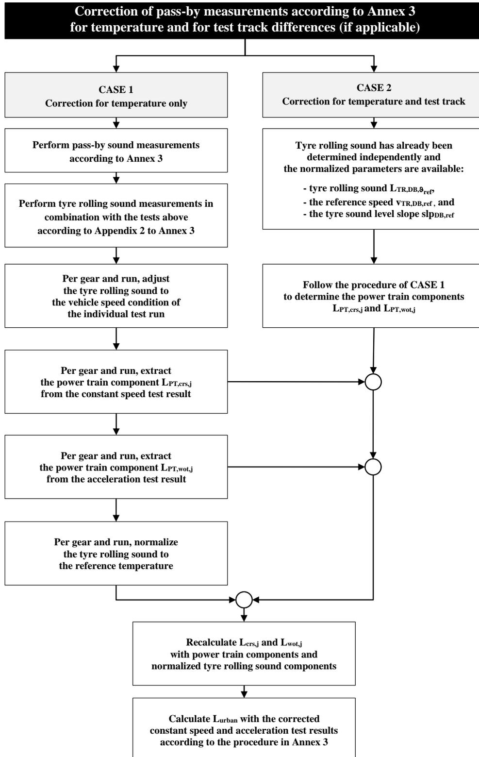
Figure 2-1: Flowchart for vehicles tested according to R51.03, Annex 3 – Correction of pass-by measurements for temperature and test track, if applicable. Flowchart from [GRBP, 2021a]
