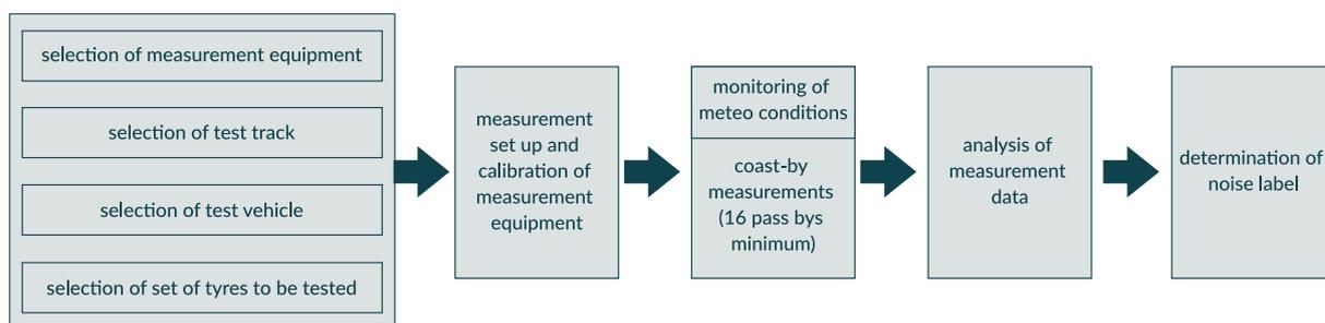
Figure 2-2: Schematic representation of the noise labelling procedure.
