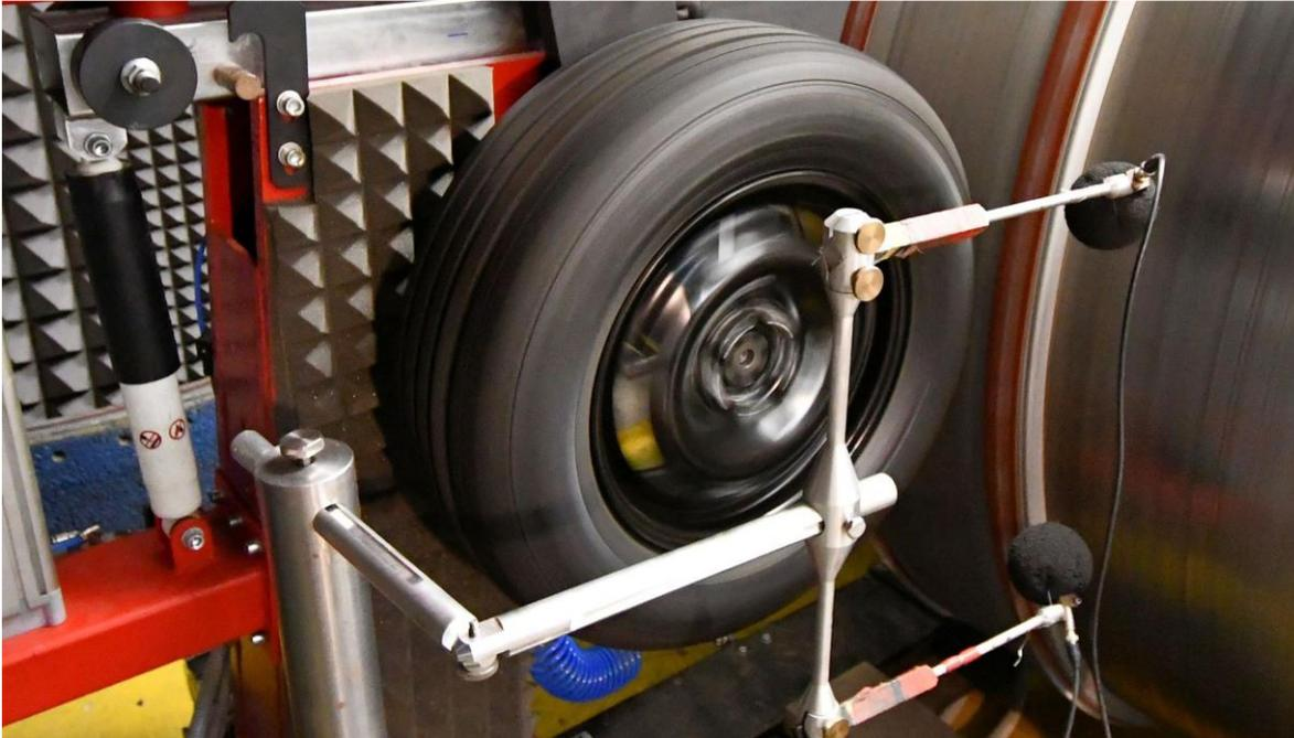
Figure 4-2: The laboratory drum facility at the GUT in Gdansk. The drum diameter is 2.0 m. An overview above and a zoom-in on the tyre/drum contact area below. Note the position of the microphones.
